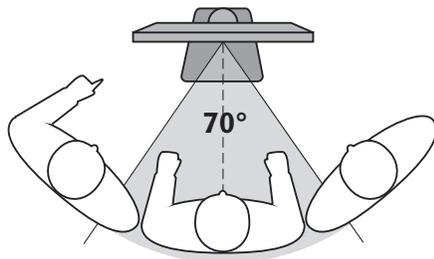
*Conventional LCD technology: colors and contrast values change substantially when looked at from an angle*
