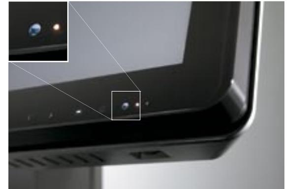
*Continuous DICOM P14 compliance under changing lighting conditions with integrated Ambient Light Compensation sensor*
